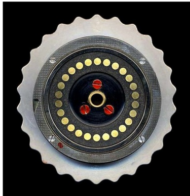
The left side of an Enigma rotor, showing the flat (plate) electrical contacts. A single turnover notch is visible on the left edge of the rotor.
